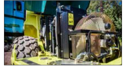
Accessible engine compartment and battery location
