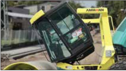
Tilting cabin for safe and easy maintenance and service
